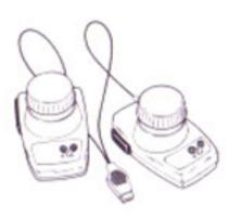
Use your Paddle Controllers with this ATARI® Game Program™ cartridge. Be sure the Paddle Controller cable is firmly plugged into the LEFT CONTROLLER jack at the back of your ATARI Video Computer System™ game.
